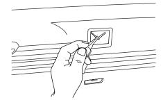
• For vehicles without power liftgate, pull the lock/unlock lever to the right (drivers side).
